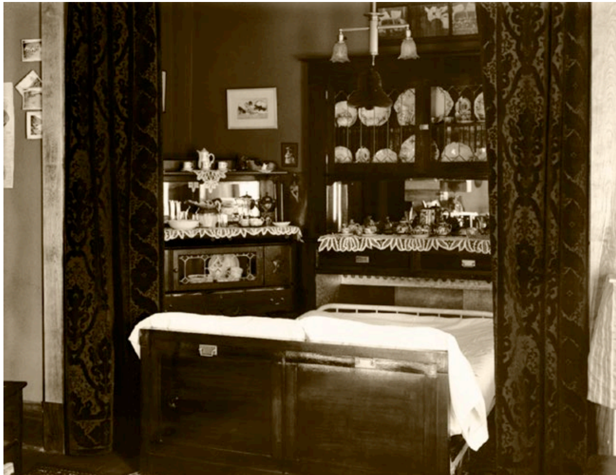
This 1908 photograph shows a “disappearing” Murphy bed in the interior of the new Woodruff Apartment building. During the day the bed could fold into the wall and the room could be used as a dining area or study. Note the velvet curtains and leaded glass sideboard. Courtesy Utah State Historical Collection, MSS C-275, #09969, Shipler Collection.
